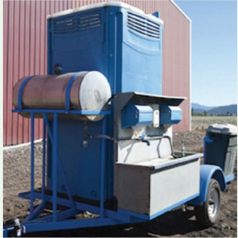
Additionally, when applying a pesticide that requires protective eyewear, 1 pint of water must be immediately available to each handler (applicator) in a portable container. It could be mounted on the vehicle, on the applicator's person, or otherwise made immediately available.
